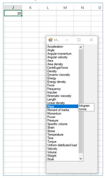
The desired unit can be selected either by typing the first letter or arrowing up/down and then pressing enter. 'kg' or 't' is displayed.
