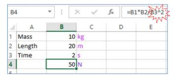
If cell B4 has dependent cells, the error message is repeated at all dependent cells and is cleared at all dependent cells when the formula error is corrected.
