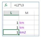
For the purposes of calculating dependent formulae, the quantity is treated as 1 million m2. Eg
