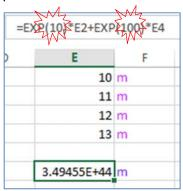
An error in the non-EXP parts of the formula is treated in accordance with the usual analysis eg mixing kg and m at cells E2 and E4:-
