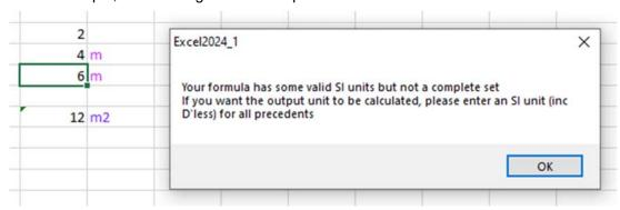
and the dependent unit is deleted (because a formula must have a full set of valid SI units for an output unit to be calculated).
