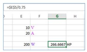
Because G5 contains a formula, not a hard entry, revision to the original inputs flows through to the non-SI unit
