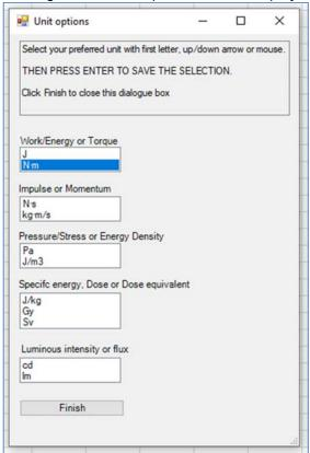
For each quantity, the preferred unit can be selected with mouse, up/down arrow or first letter. After selection, 'Enter' will bring up message to ask for confirmation that the unit is to be stored.
