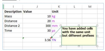
Н K M **Description Value** Unit 10 kg Mass Distance 20 m 300 mm Distance 2 30 Jus Time You have added cells with the same unit but different prefixes =J2\*(J4+J3)/J5^2 GN Excel2024\_1 X The cell at Sheet1!J3has the same dimensions as the cell at Sheet1!J4but a different prefix If your formula does not allow for this it will be numerically incorrect
