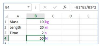
Now the add-in will automatically calculate the unit of the output quantity and write it to the adjacent cell, C4.
