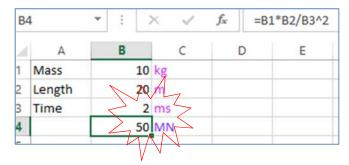
The add-in provides a powerful check on the correctness of all scientific and engineering formulae entered to an Excel worksheet.
