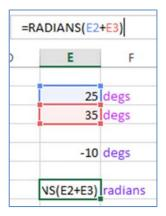
When included in a wider formula the output of RADIANS is treated as a dimensionless quantity. Inverse trigonometric functions are treated as (dimensionless) radians eg
