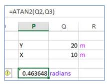
If the arguments are included as values in the formula eg =ATAN2(2,1), the add-in does not calculate an output unit but if used in a wider formula is correctly treated as dimensionless eg.
