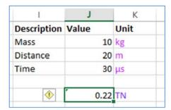
A second type of error picked up by the add-in might simply result in an invalid physical unit. For instance, if the user incorrectly types 3 for the time exponent instead of 2 (an easy keyboard error to make), Excel does not care that this makes no physical sense and returns a value for the formula at J6.
