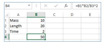
If the user enters the formula = B1\*B2/B3^2 at cell B4, the quantity calculated is a force in Newtons. But if the user mistakenly enters = B1\*B2/B3^3, Excel still calculates a valid number but the quantity is not a force. Only a rigorous check of the worksheet would find this error.
