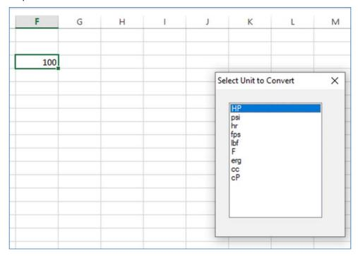
Typing first letter followed by Enter enters the selected unit in G3 and also enters the konversion formula in H3 and the appropriate SI unit in I3:
