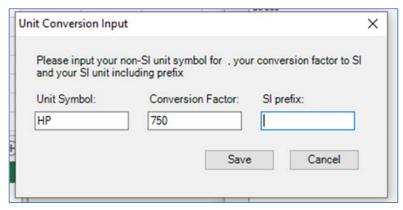
If the user wants the konversion to be from HP to kW, the prefix "k" is entered in to the 'SI prefix box BUT in this case the Conversion Factor value would be 0.75 (or whatever level of accuracy the user requires)
