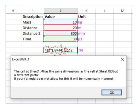
A warning comment is added to the cell and a unit is displayed based on the prefix of the <u>first</u> <u>distance</u> specified in the formula.
