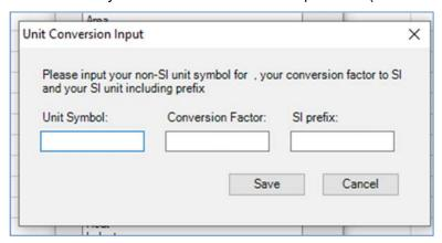
In the 'Unit Symbol' box, the user types their chosen symbol for a non-SI unit eg "HP" for horsepower. Tab moves to 'Conversion Factor' where the user enters the numerical value converting HP to the SI unit Watts:
