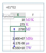
If the unit of 'MJ' at cell E3 was deleted, the calculated unit of 'TW' at E7 would not be correct. The add-in therefore prevents the user from deleting any units calculated by the add-in:
