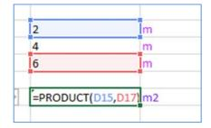
With valid units at D15 and D17, the output unit is m2. If D15 is selected and Ctrl Alt d is invoked, the add-in first asks the user to confirm the deletion.
