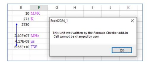
The user has attempted to delete the unit at F3 and is presented with a message saying that this unit cannot be changed by user. Upon clicking 'OK' the message is removed and the unit is reinstated:
